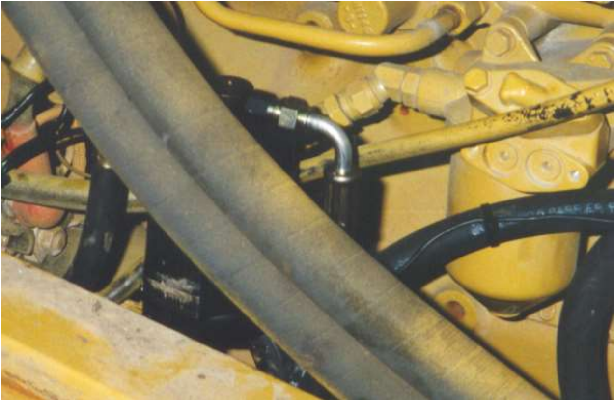
View showing drier and hoses in place.
