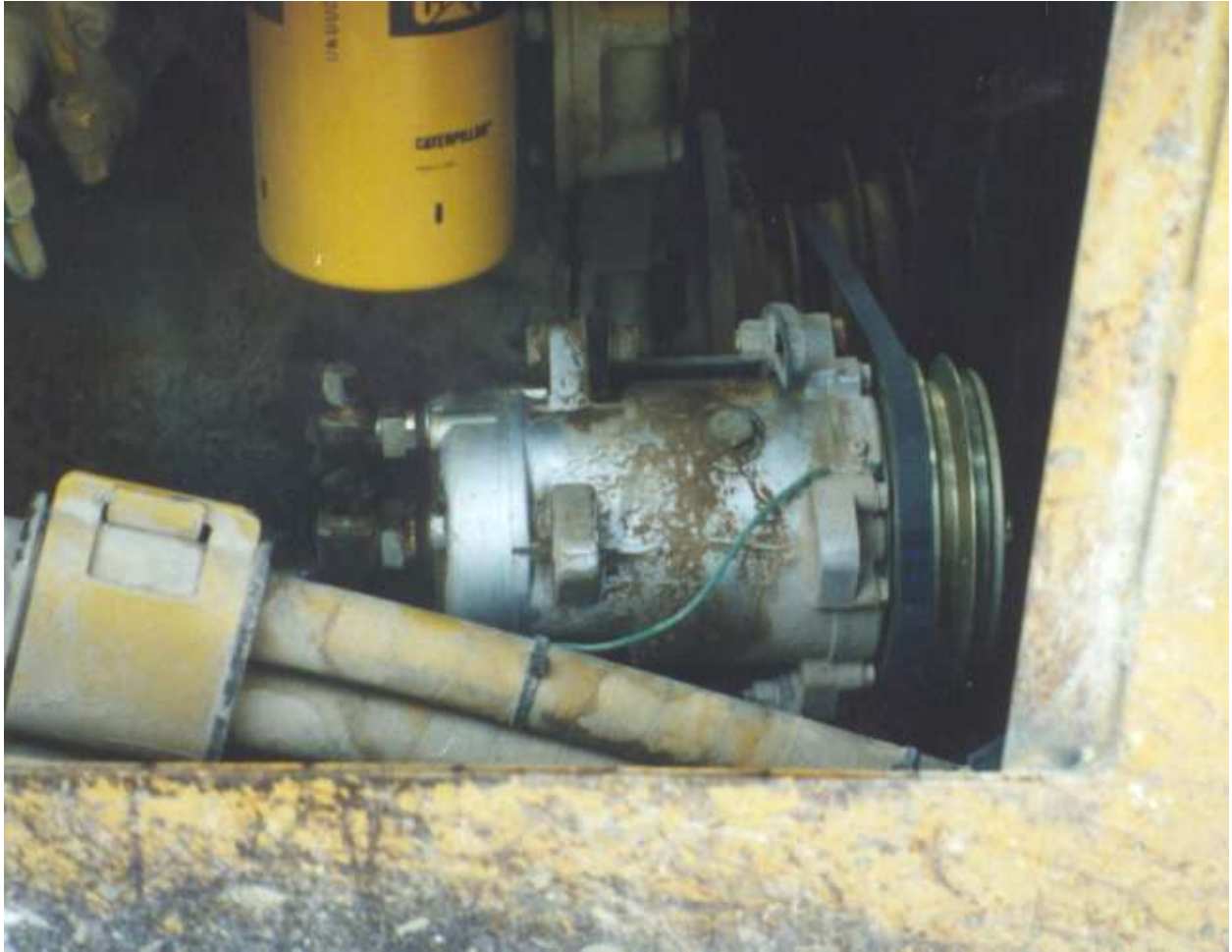
Compressor mounted in place - new style compressor.
