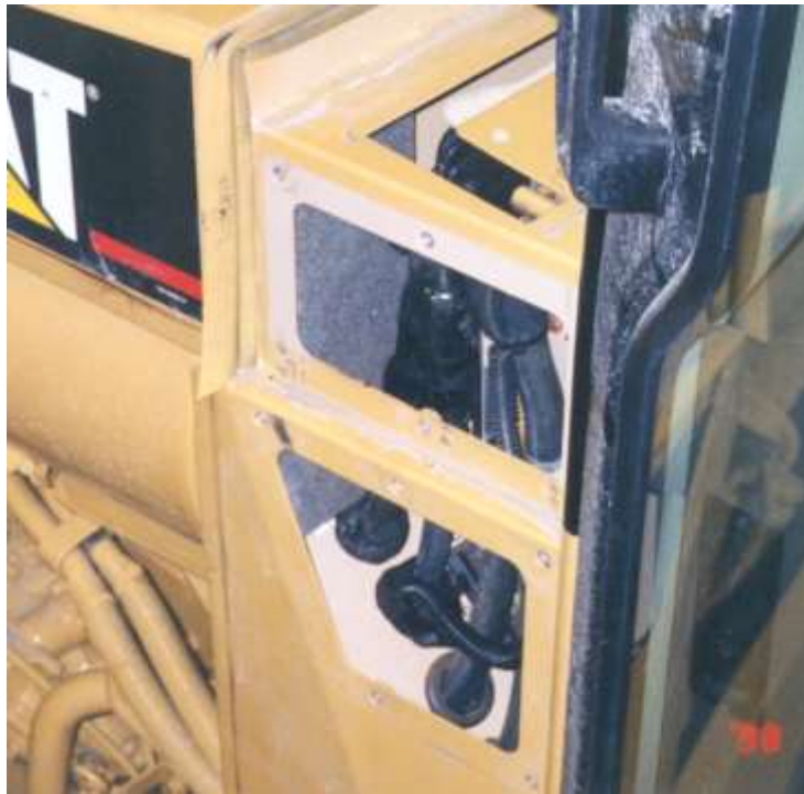
Evaporator assembly showing hoses.
